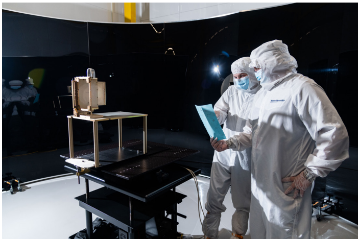
Instrument under test mounted on a rotary table.
