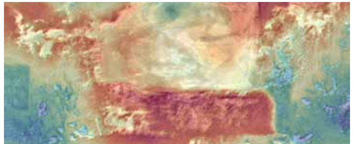
Digital Surface Model (blue is 0 m, red is 3 m) overlaid on a true-color composite of a 30-minute, 30-acre collection capturing a Helicopter Landing Zone (HLZ) at 3 cm/pixel.
