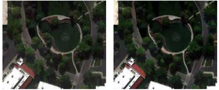
Pan-sharpened RGB (left) and true-color composite (right) showing a portion of a 30-minute, 30-acre collection capturing an urban environment at 3 cm/pixel.
