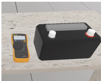
Battery Voltage Test Demonstrates measuring the voltage of a DC battery using a multimeter.
