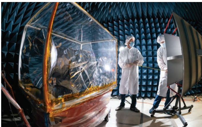
SDL engineers environmentally test the AWE flight model.
