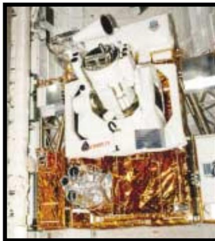
**Top: Engineers at SDL tape thermal blanketing on the SABER infrared telescope in preparation for final testing**
