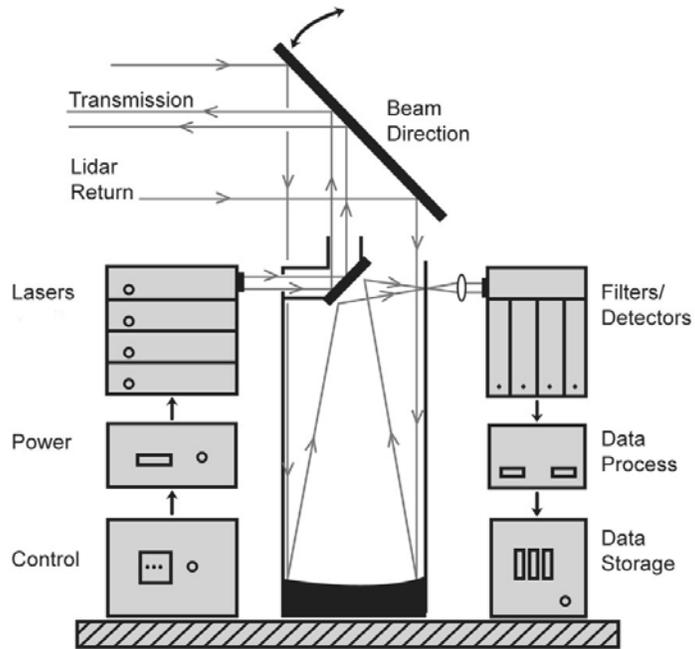
Figure 1. Schematic of AGLITE lidar design and construction.
